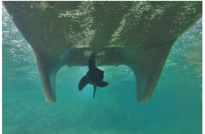
Orientable electric pod, protected by the keels
