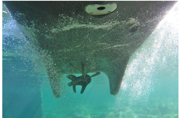
Muscular propeller and orientable electric pod
